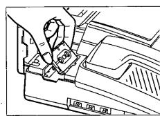
Insert the microcassette tape into the compartment with the full reel to the left.
