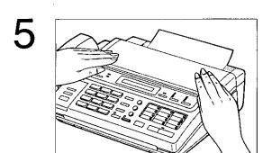
Close the paper compartment cover carefully by pressing down on both ends gently.
