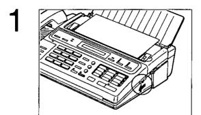
Slide the FRONT LID OPEN lever forward to open the document feeder unit.
