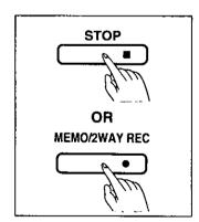
To stop recording, press the STOP button or the MEMO/2WAY REC button again.
