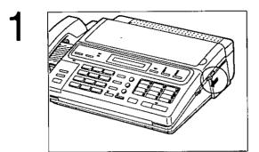
Slide the BACK LID OPEN lever forward to open the recording paper unit.
