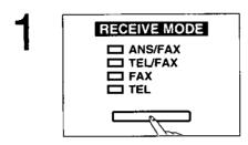
Press the **RECEIVE MODE** button until the ANS/FAX indicator lights.
